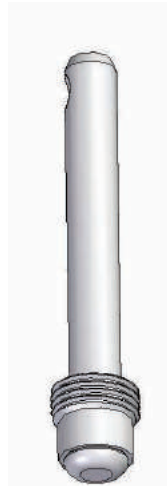
Soft-seat Stem Repetitive shut-off for gas
